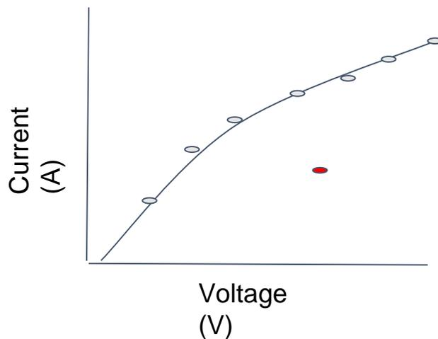
We can see that as the voltage increases so does the current but the rate of increase is not consistent. Therefore we would not get a straight line on a line graph. The line graph above shows that there is a trend; as the voltages increases, the current increases but the rate of increase becomes slightly less.
