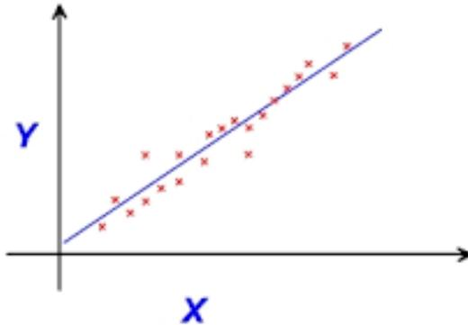
A line of best fit is shown above. A line of best fit is used to help identify any values that have been measured incorrectly.
